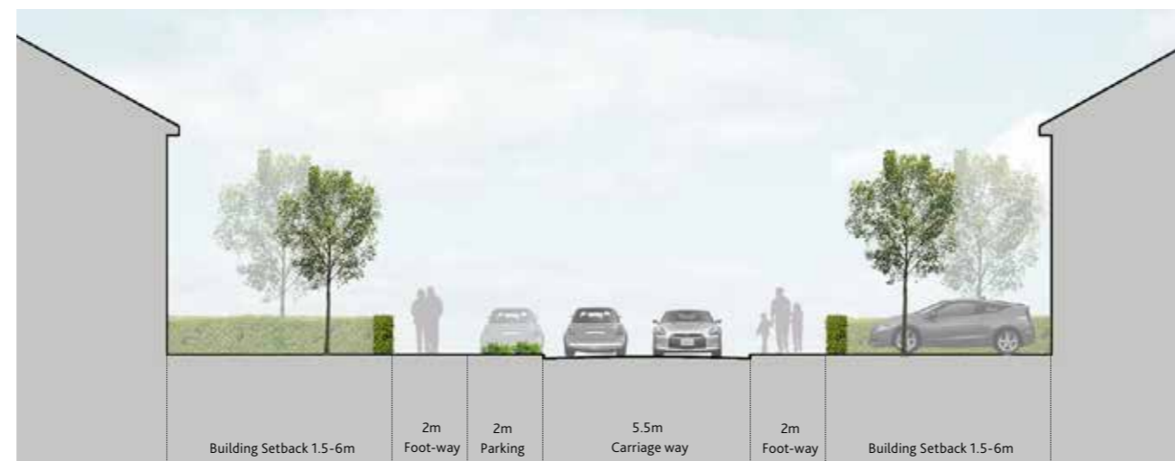
FIG.52: SECONDARY STREET SECTION WITH ON-STREET PARKING BAYS
