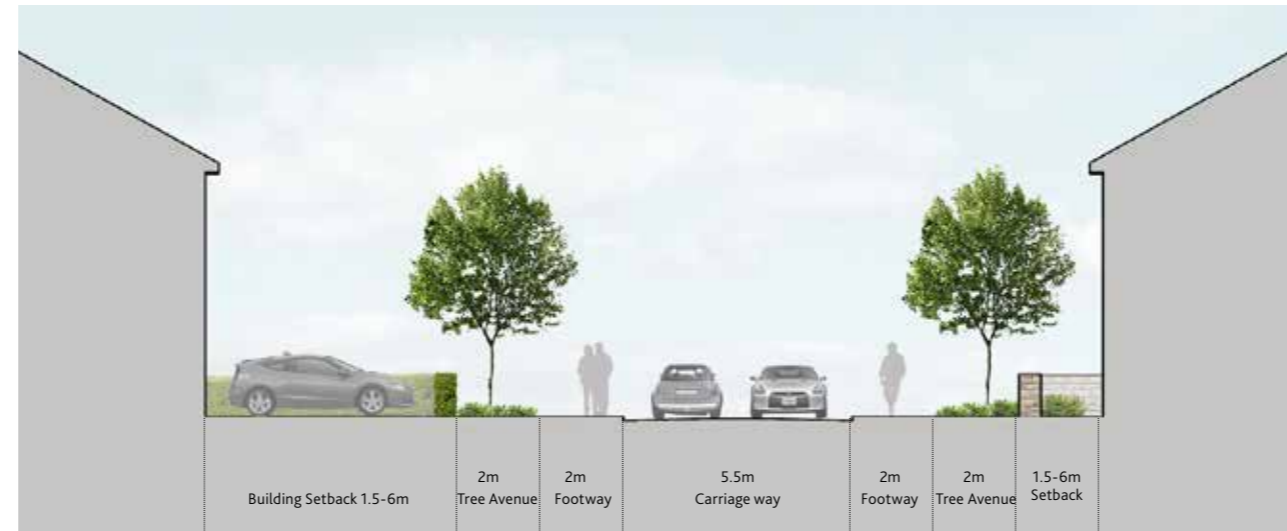
FIG.49: ST1.B PRIMARY STREET (AVENUE) TYPICAL SECTION
