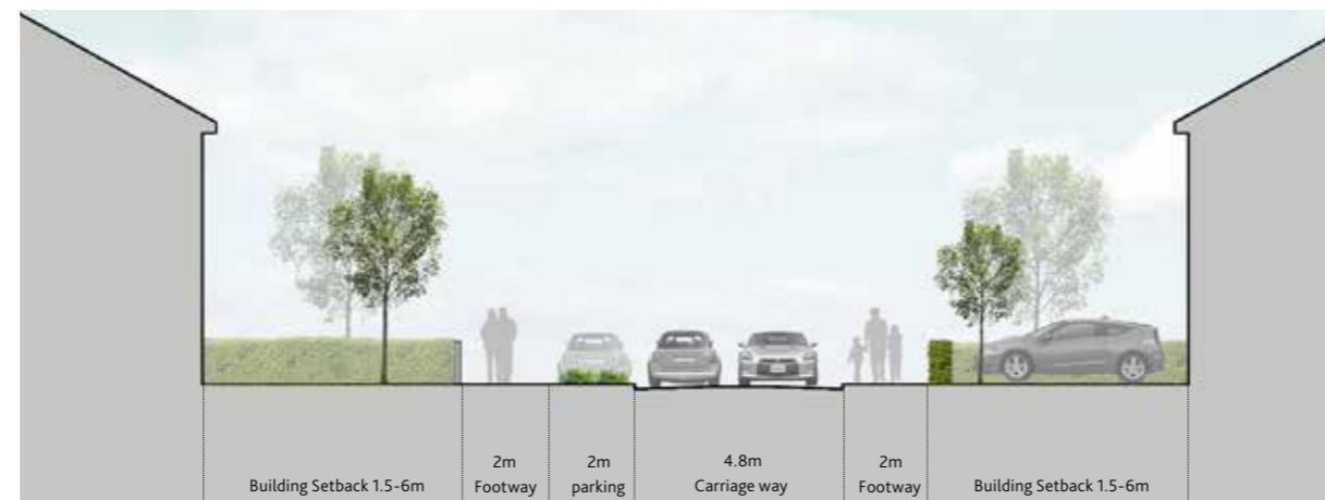
FIG.54: TERTIARY STREET SECTION WITH ON-STREET PARKING BAYS
