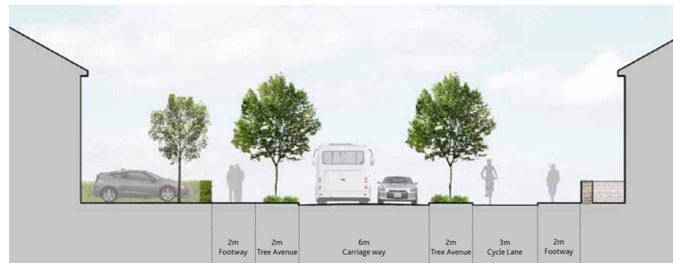
FIG.43: SECTION OF THE BUS-COMPATIBLE PRIMARY STREET SHOWING THE 3M SEGREGATED CYCLE LANE
